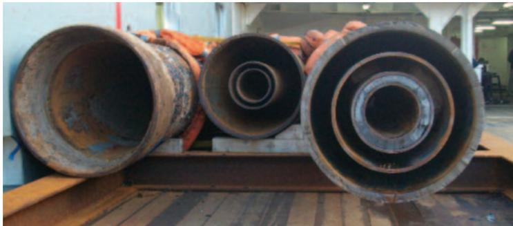
Figure 4-1 - Subsea well casings cut using AWJ based cutting tools, [1]
