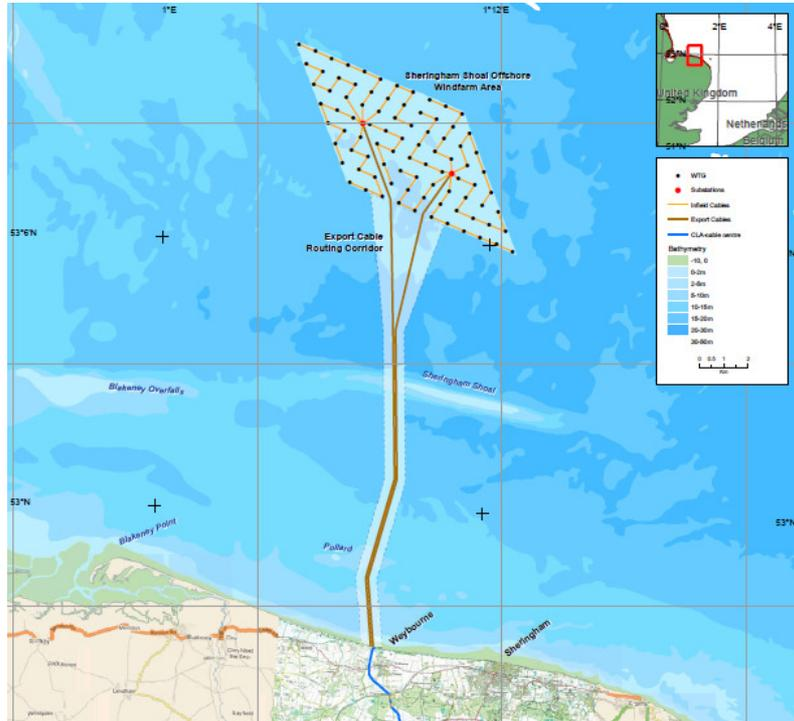
Figure 4.7 Route of the marine export with corresponding landfall drill and junction pit
