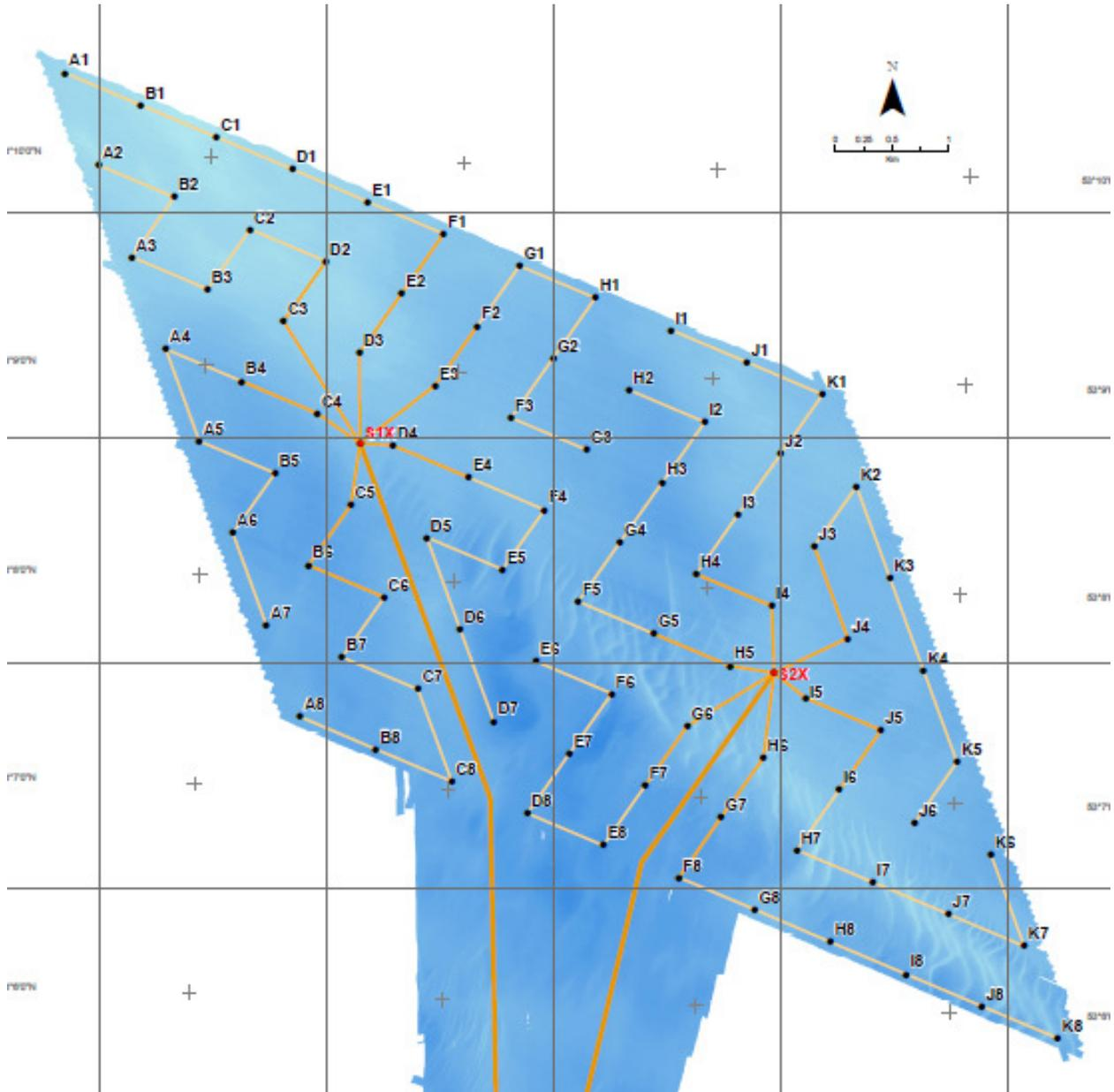
Figure 4.8 Layout of the in-field marine cables
