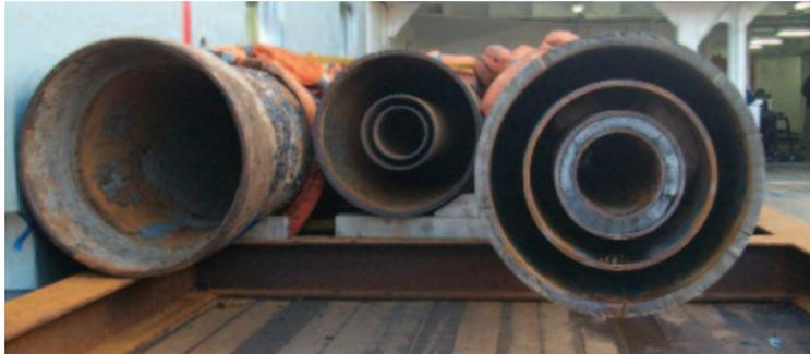
Figure 4-1 - Subsea well casings cut using AWJ based cutting tools, [1]
