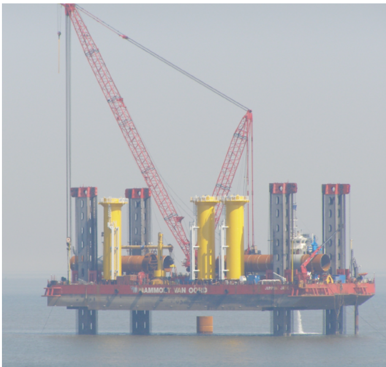
Figure 4.5 Foundation – example of possible vessel
