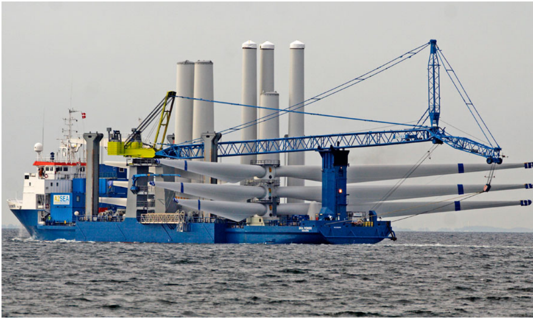
Figure 4.3 Example of possible transportation of WTGs
