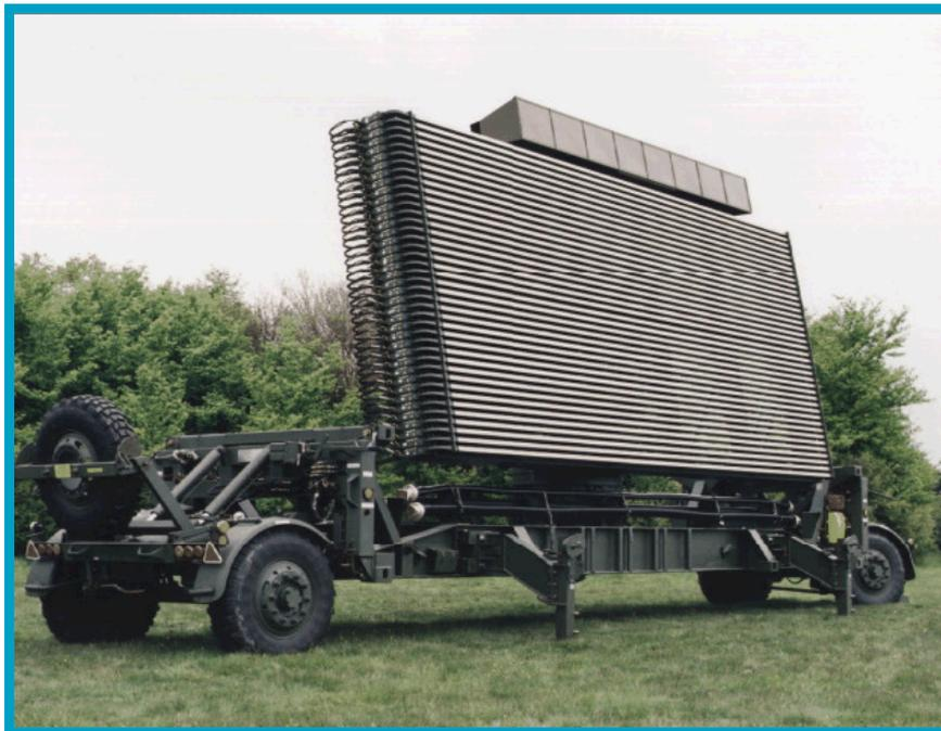
*Plate 16.1 The antenna for the AR327 air defence radar (Type 101).*
