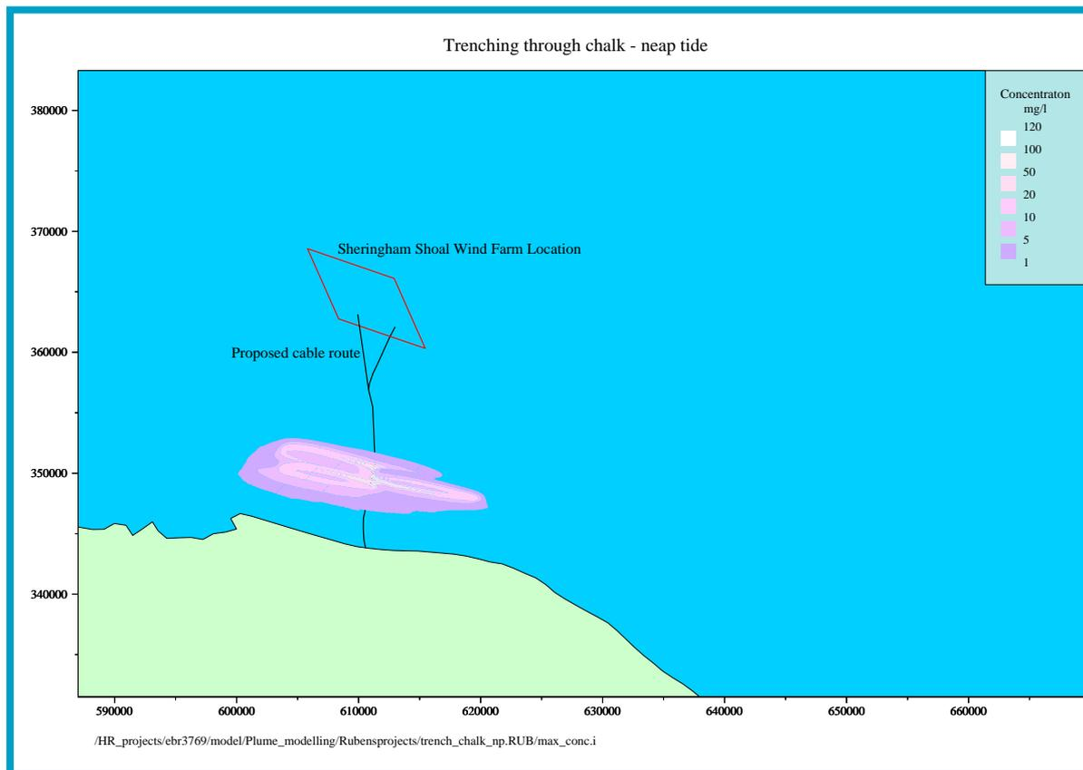
Figure 7.6 Peak suspended solids predicted to occur over neap tides for installation of export cables via trenching
