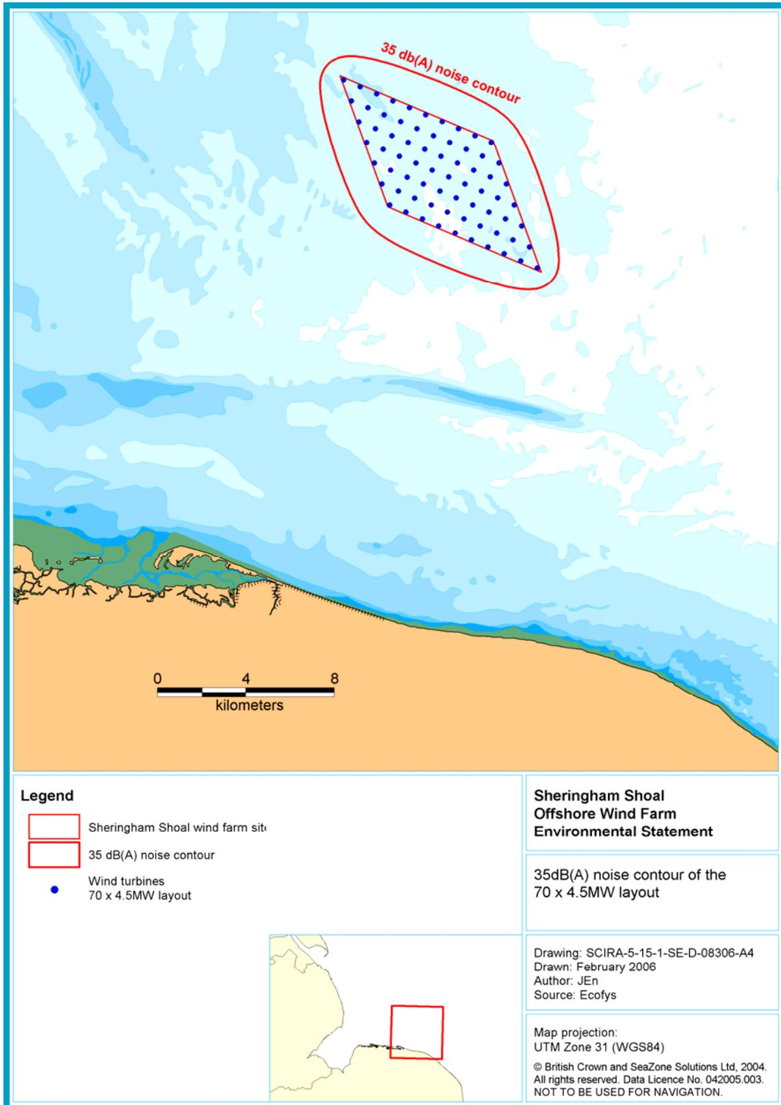
Figure 2.15 35db(A) noise contour of the 70 x 4.5 MW layout.
