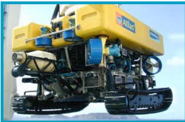
Plate 2.25 Jet equipped remotely operated vehicle
