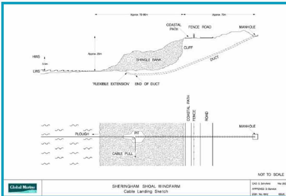
Figure 2.19 Cable Landing Illustration
