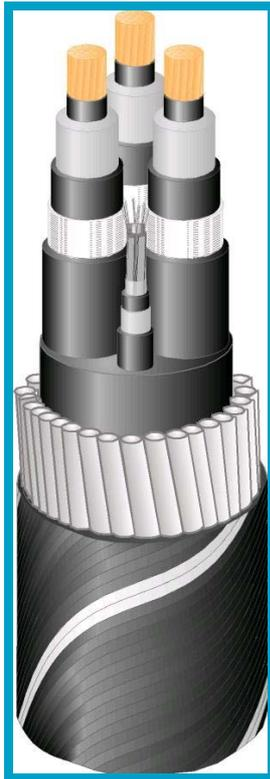
Figure 2.3 Typical 3 Core Copper XLPE Armoured 132 kV Subsea Cable with fibre optic cable (Courtesy of ABB)
