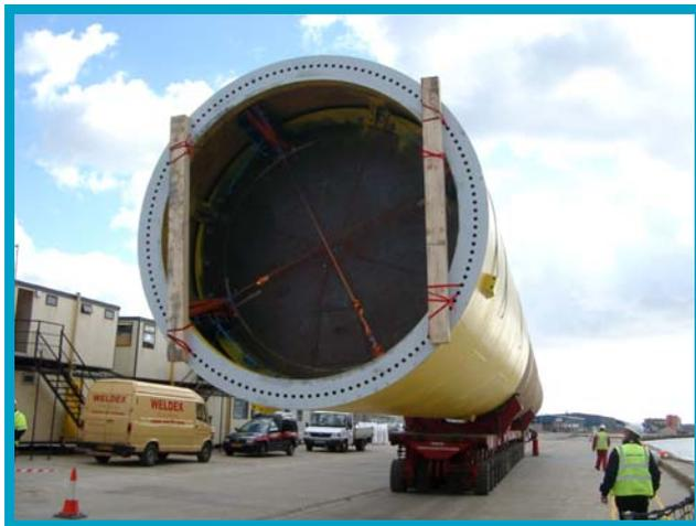
Plate 2.9 Pile, complete with tower flange, ready for loading
