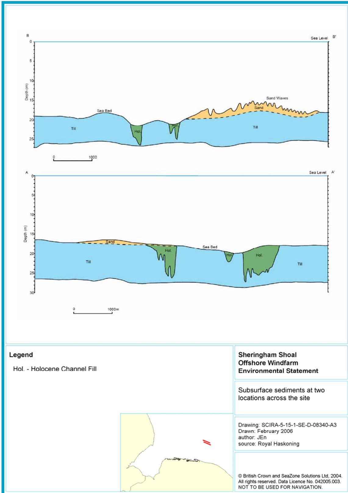
Figure 2.9 Subsurface sediments at two locations across the site
