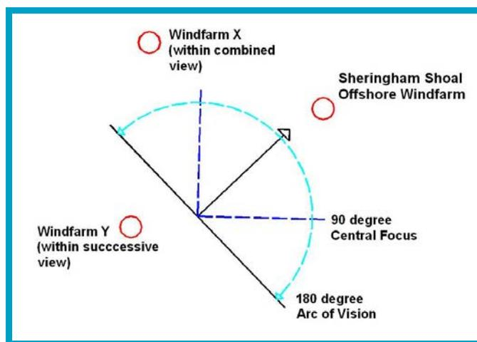
Figure 13.4 Illustration of Combined and Successive Impacts (Source: ERM)
