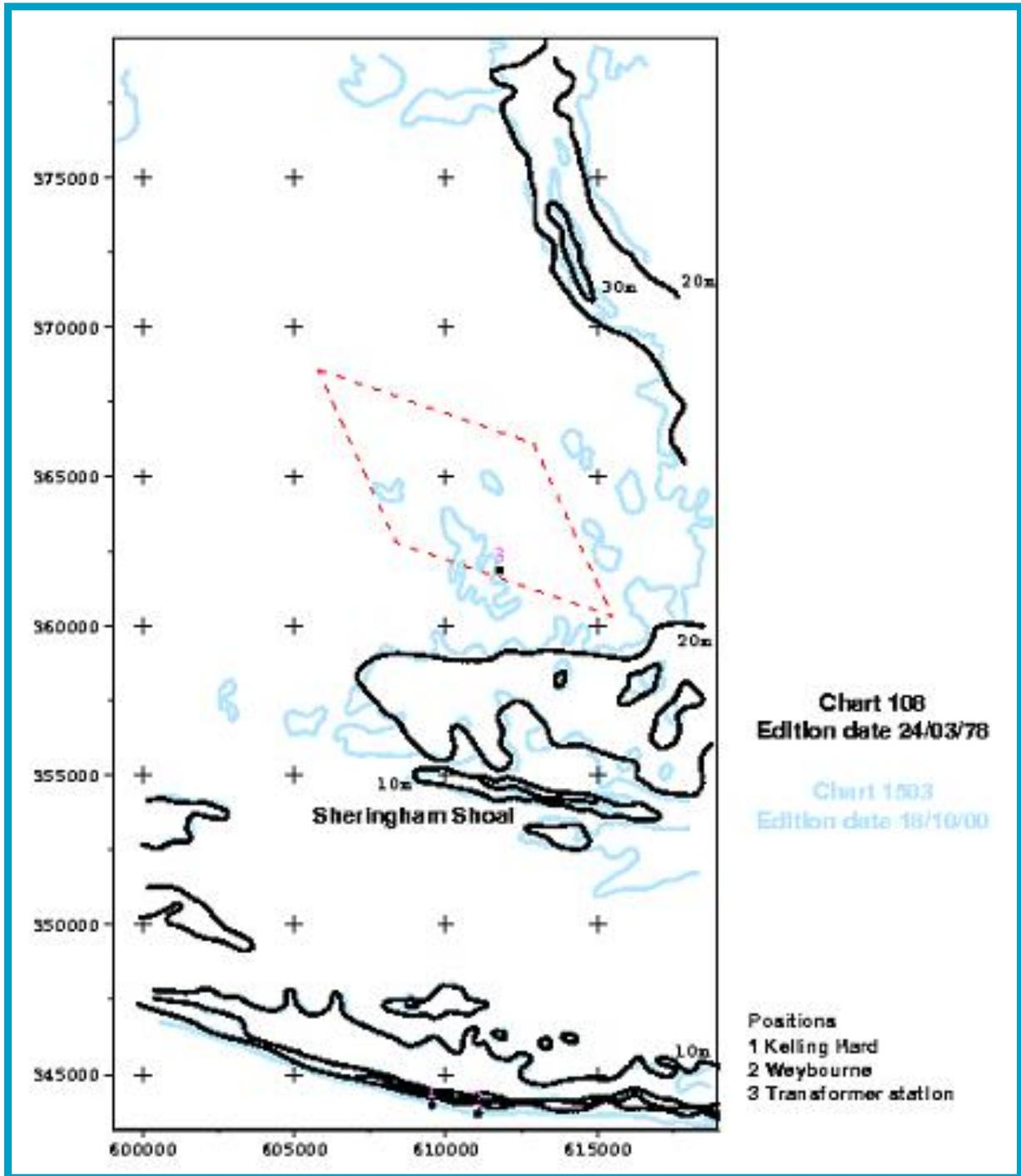
Figure 6.8 Comparison of landfall seabed contours
