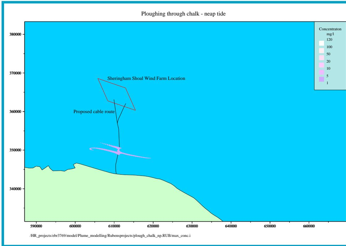
Figure 7.4 Peak concentrations of suspended solids during neap tides for installation of export cables using the plough method
