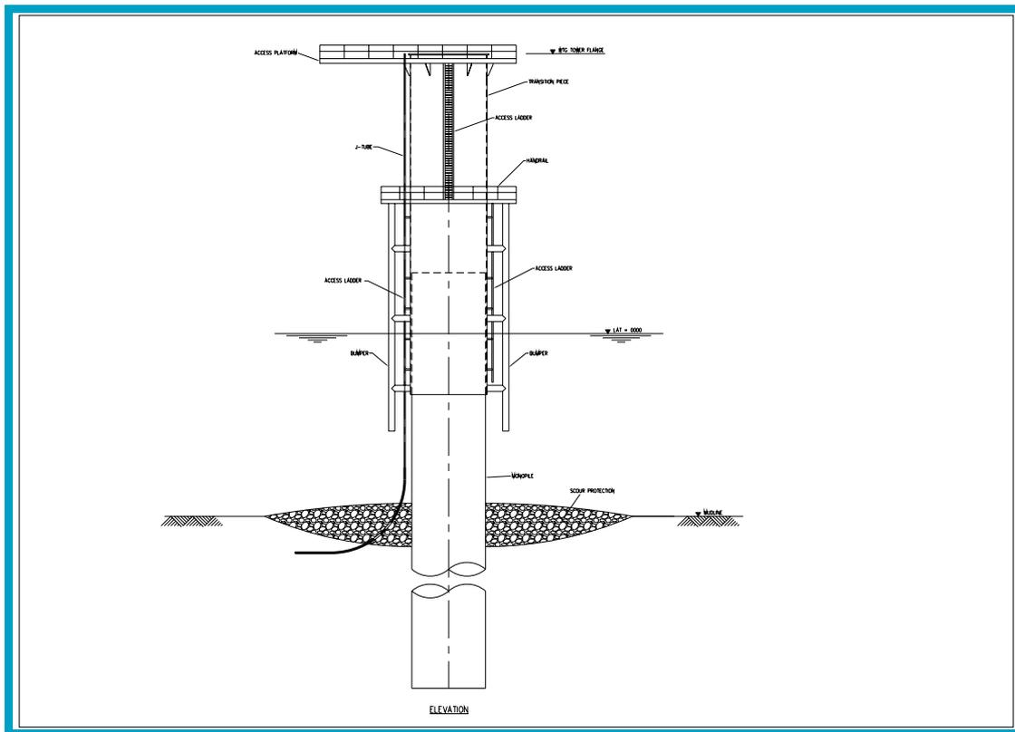
Figure 2.10 Indicative design of a mono pile foundation.
