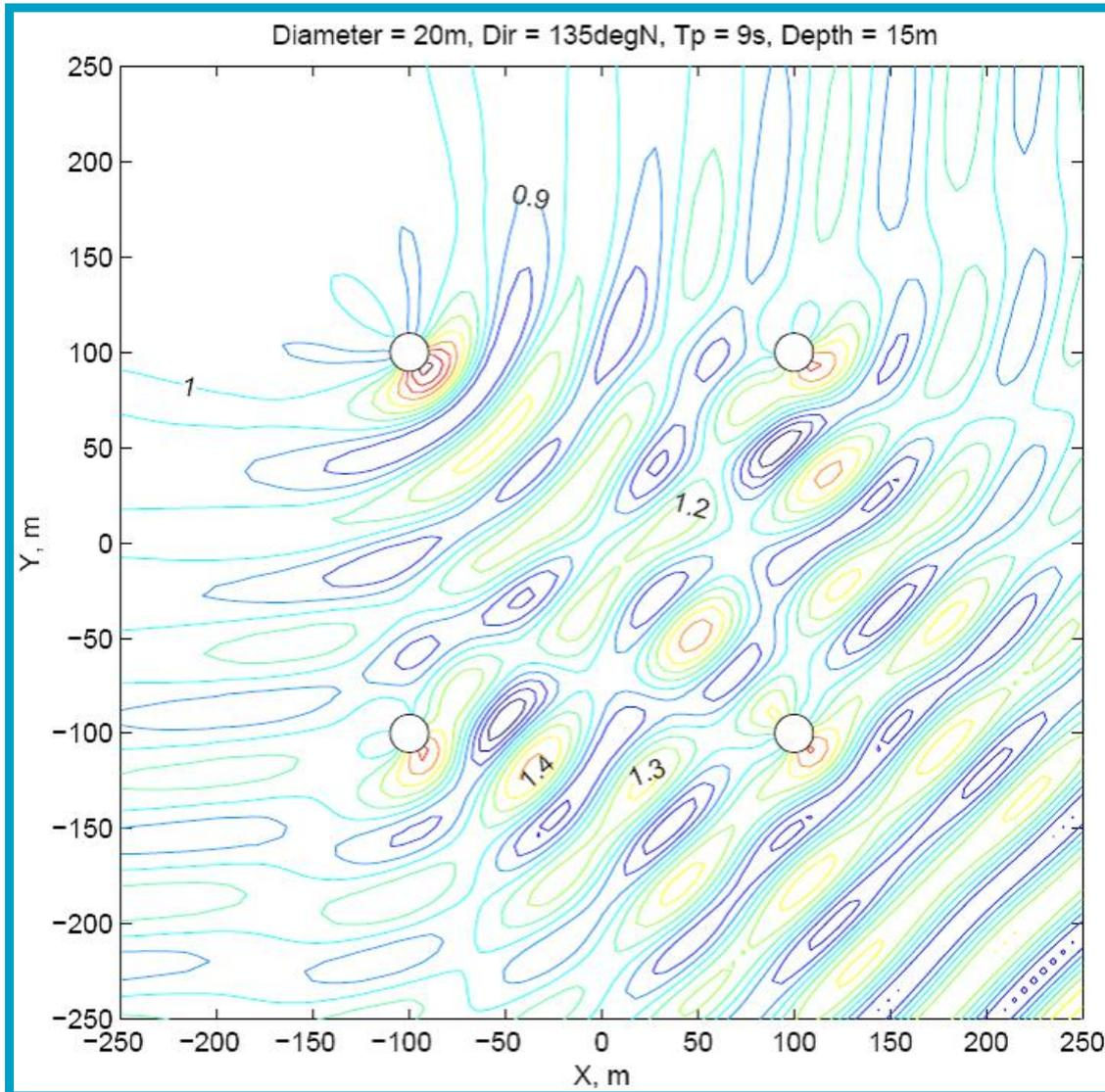
Figure 6.20: Wave scattering from 20m diameter cylinders at 200m spacing Source: derived from Ohi et al (2001)
