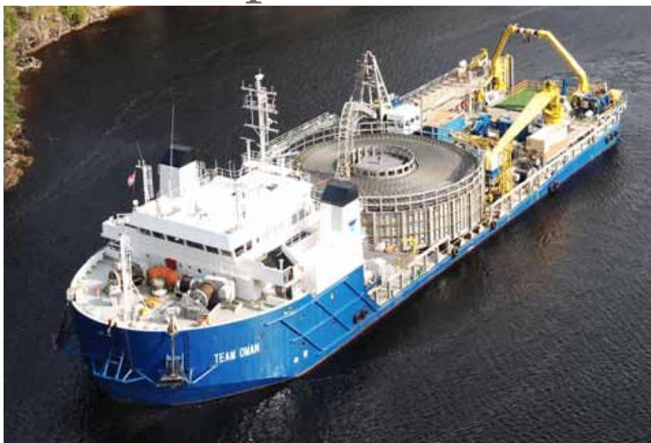
"Team Oman" loaded up with the cables bound for the Sheringham Shoal project.
