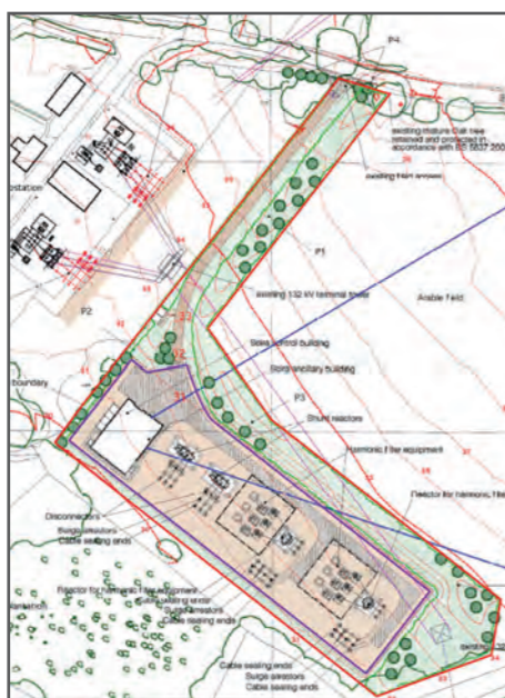
New equipment positioning at the Salle onshore electricity substation
